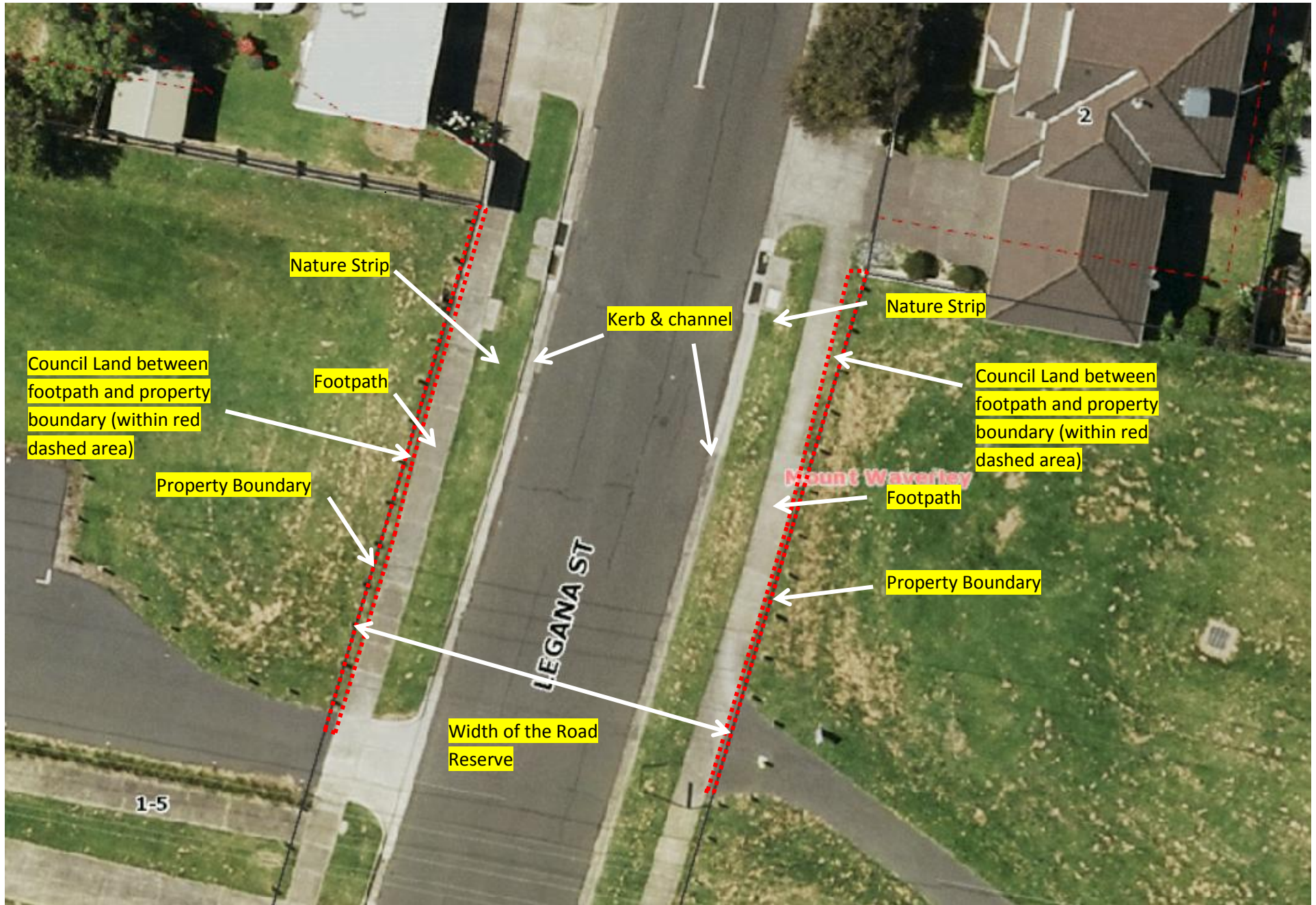
Diagram showing the Road Reserve and how it may affect construction along the front of your property (City of Monash)
