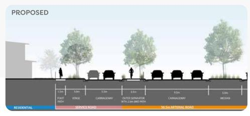
Figure 7. An example of a cycle path within the outer separator (where appropriate widths permit), which has no impact on service road traffic flow, and includes including low planting and a traffic barrier for safety. Cyclists would need to give way where vehicles enter/exit the service road. Example provided opposite, on Andersons Creek Road, Doncaster East.
