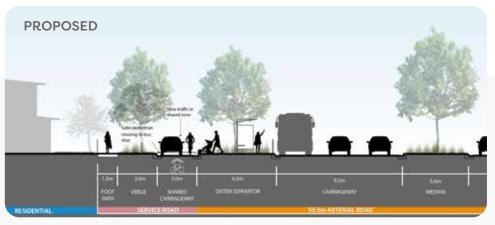
Figure 6. An example of a reconfigured service road, that could be utilised at key locations where pedestrian crossing movement should be prioritised - this example would provide traffic calming through a narrowed pavement, kerb outstands, line marking, and increased pedestrian activity.
