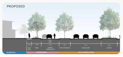
**Figure 8.** An example of a reconfigured service road showing a carriageway that supports on street parking, one way through traffic, and cycle movements in a shared road 'sharrow' environment. Regular traffic calming measures should be utilised to slow vehicle traffic on long service road lengths - options include kerb outstands, speed humps, line marking as potential options.
