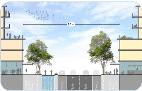
Figure 31: Area 3 – Potential Huntingdale Road section.
