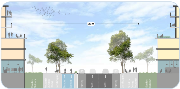
Figure 29: Area 3 – Potential Huntingdale Road section.
