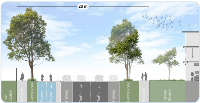
Figure 54: Area 7 – Proposed street section Huntingdale Road.
