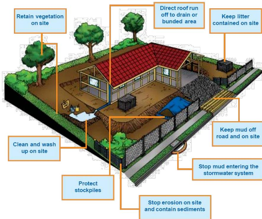
Figure 10: Stormwater will be effectively managed during construction phase according to the requirements listed in “*Keeping Our Stormwater Clean – A Builder’s Guide*”.
