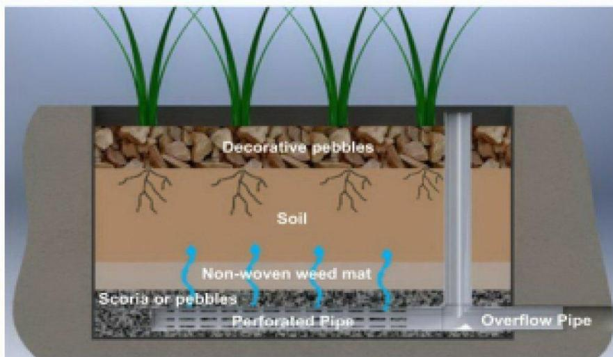
Figure 3.3 Typical Raingarden in ground for illustration purpose
