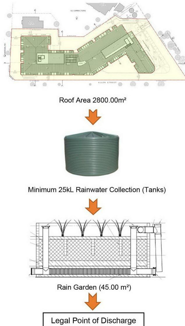
Figure 3.1 Treatment Train Schematic
