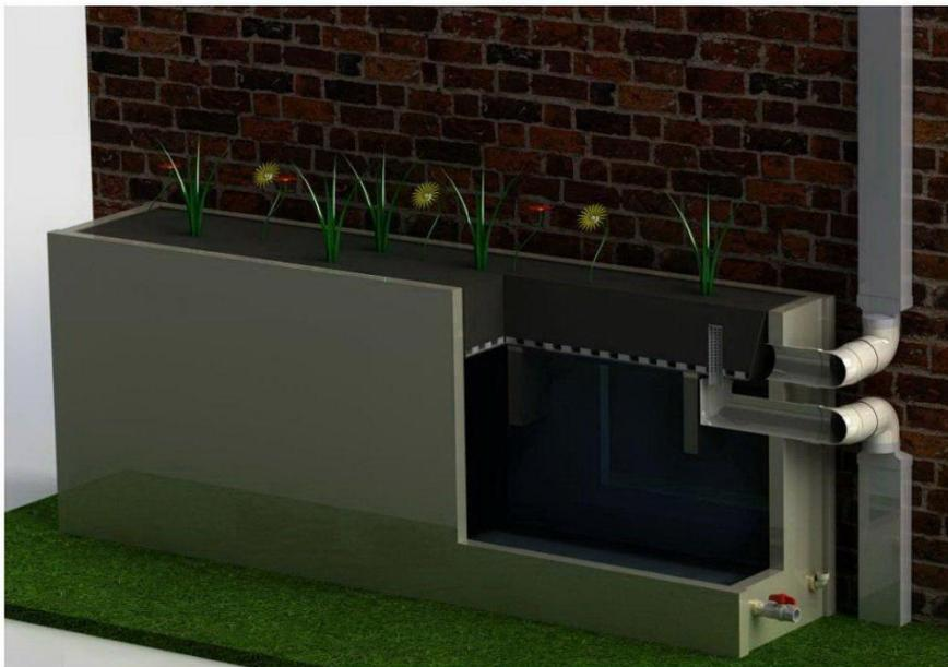
Figure 3.2 Typical Raingarden in ground illustration
