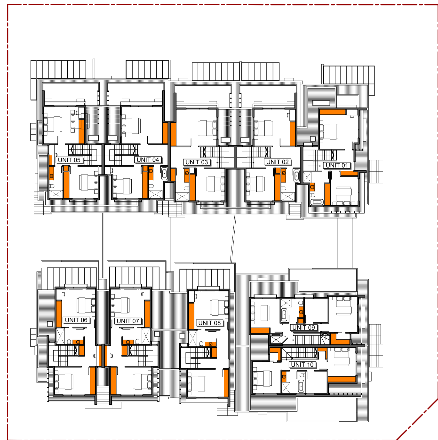
INTERNAL STORAGE - LEVEL 2 SCALE 1:200
