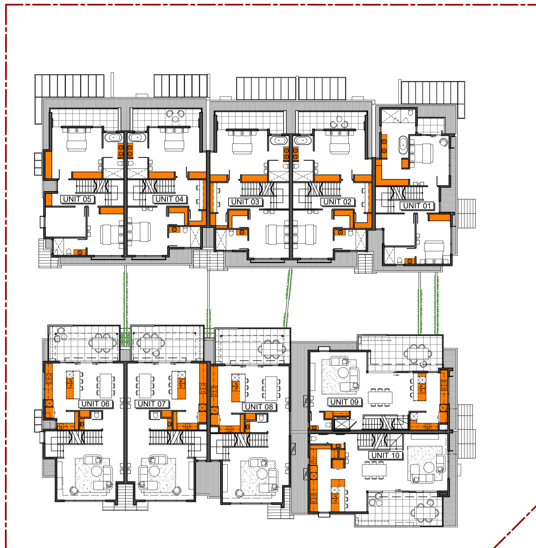
INTERNAL STORAGE - LEVEL 1 SCALE 1:200
