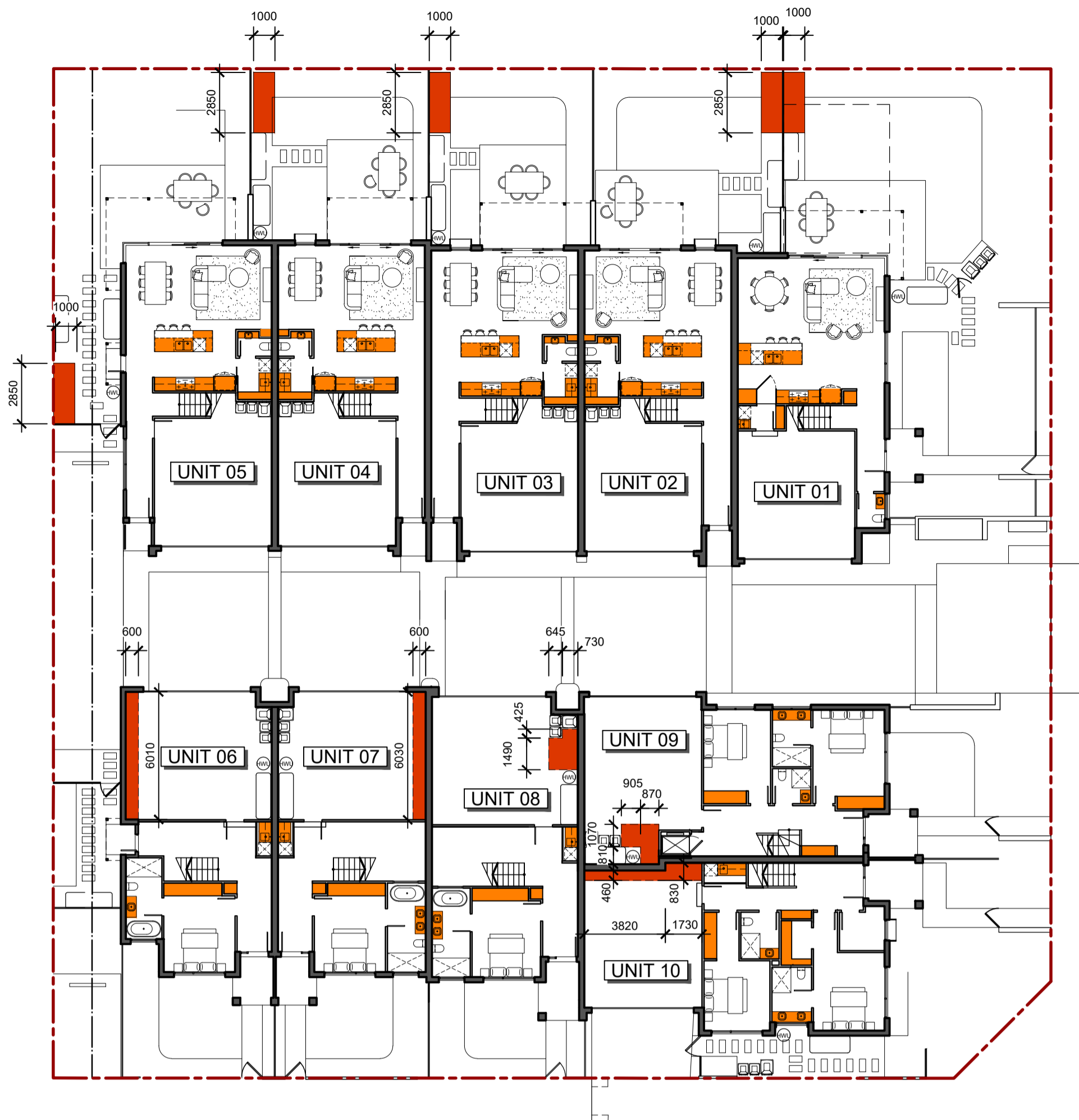
INTERNAL & EXTERNAL STORAGE - GROUND LEVEL SCALE 1:200
