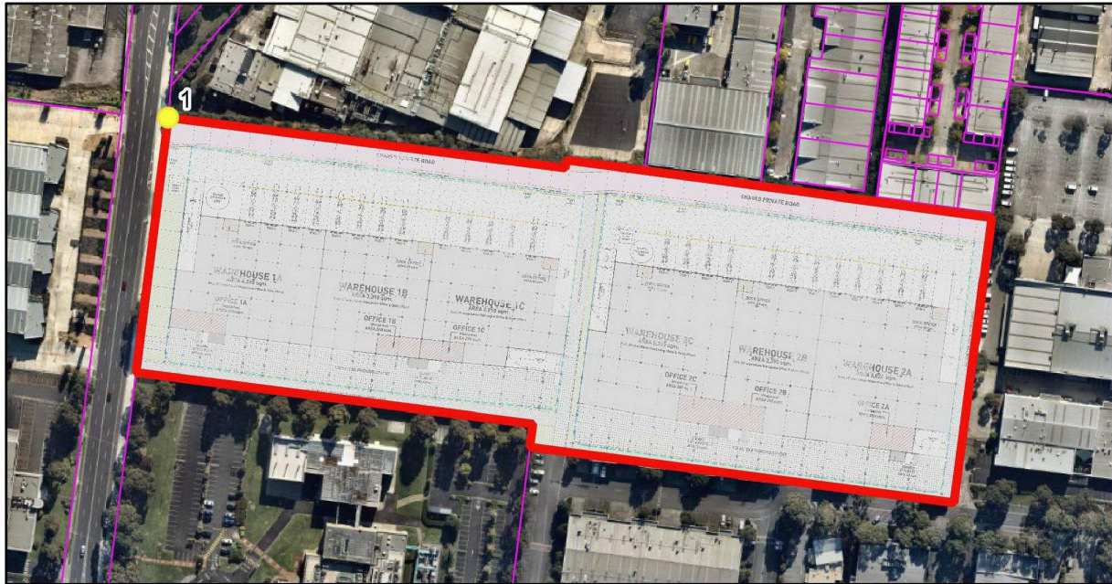
Figure 6: Developed catchment plan showing location of peak flow calculation.
