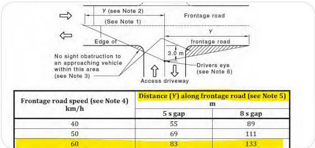
**Note 5:** These distances are equivalent to minimum gap sight distance (MGSD) for an exiting vehicle. The minimum requirement is a 5 s gap. A right turn exit into a six lane road may require up to an 8 s gap, unless the median is wide enough to shelter a vehicle leaving the driveway.
