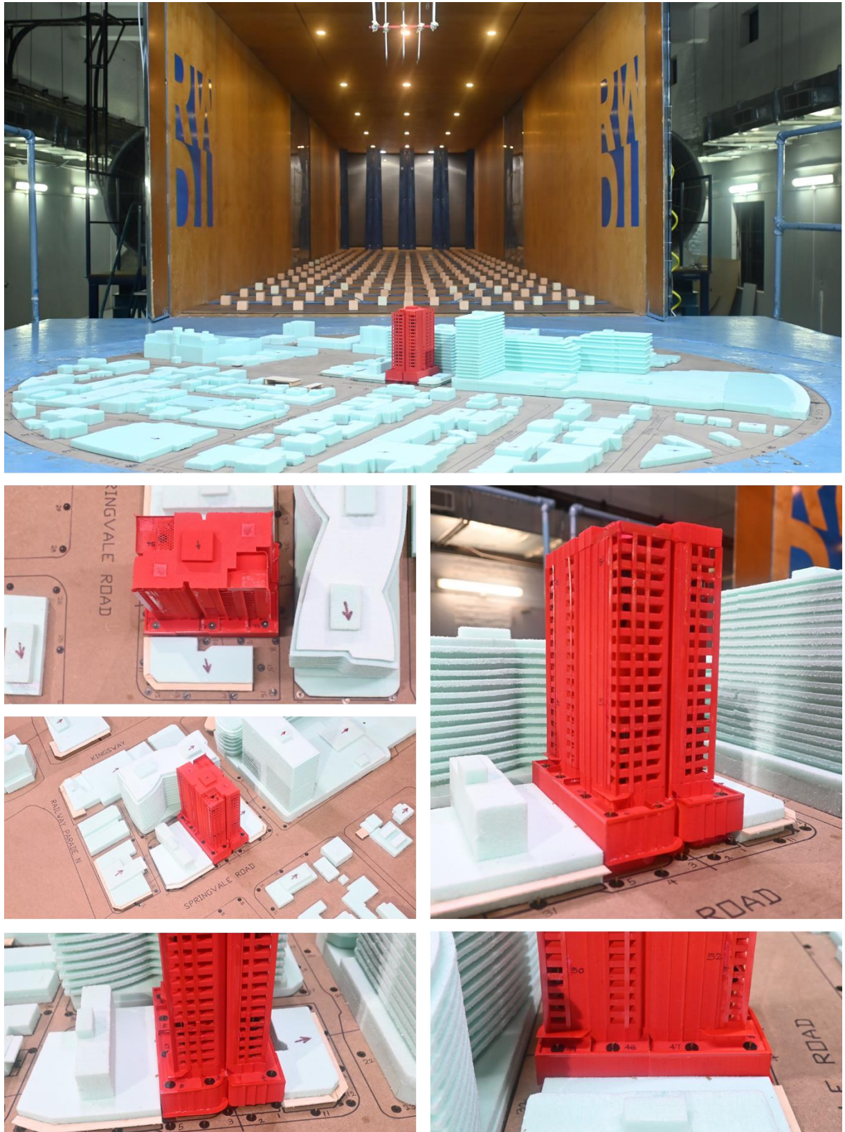
Image 2B: Wind Tunnel Study Model – Proposed Configuration
