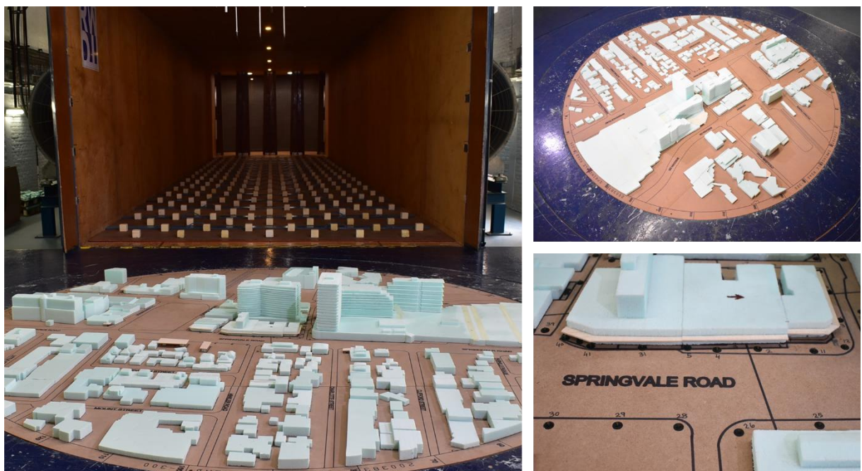
Image 2A: Wind Tunnel Study Model – Existing Configuration
