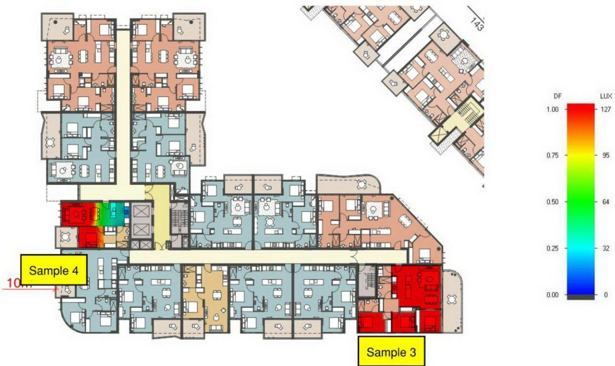
Figure 8 - Daylight Map – First Floor
