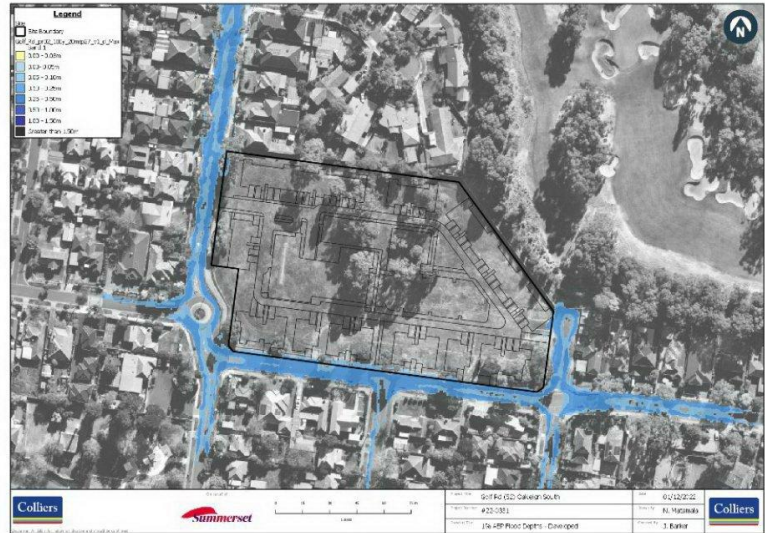
Figure 10. Mitigated Conditions 1% AEP Flood Depths
