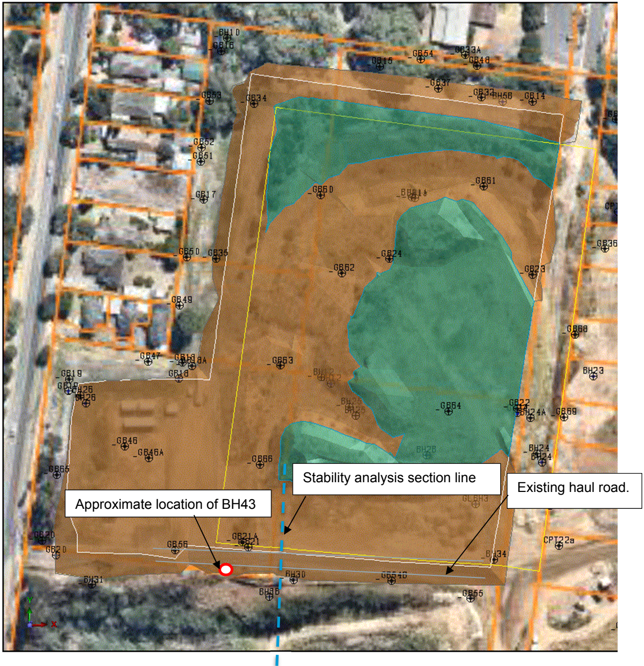
Figure 3 - Zone 1 proposed preload extending to the crest of the Zone 4 north batter
