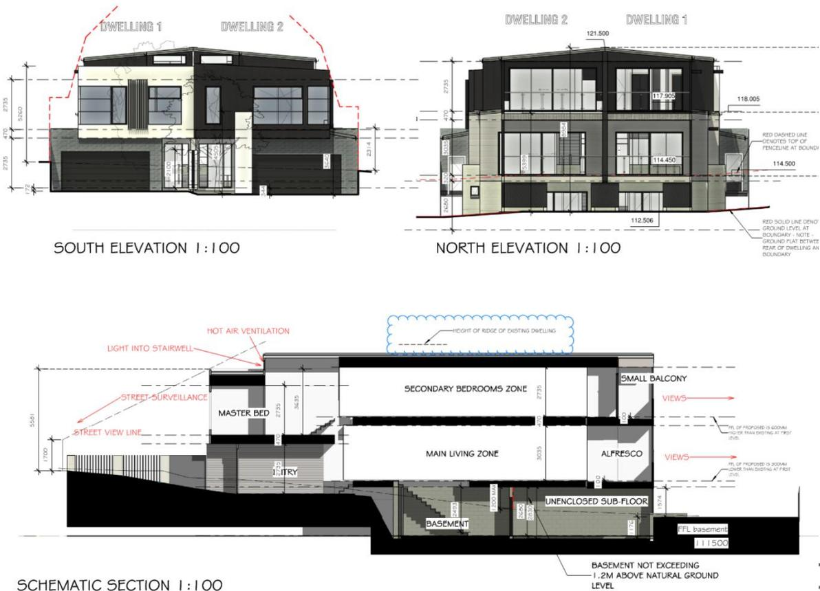
Figure 1 - Elevations and cross section of proposed dwellings.
