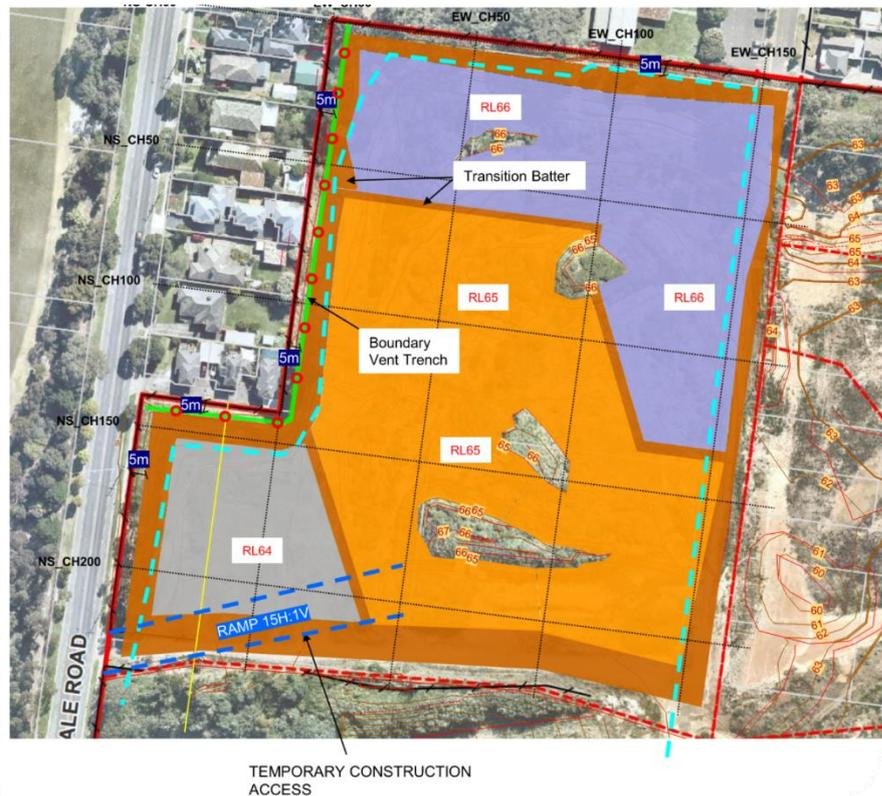
Figure 3 - Preload layout with respect to pit crest (pit crest marked in blue dashed line). Green dashed line shows the line of gas vent locations.
