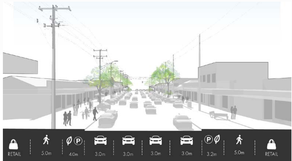
Figure 20. Clayton Road Existing Cross Section
