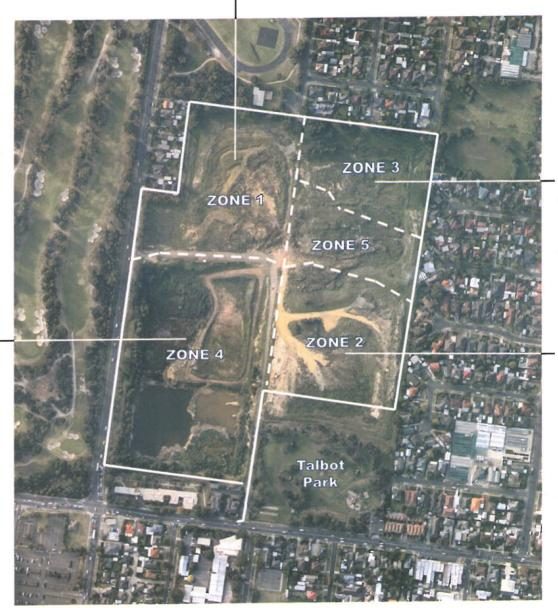
Variable Thickness of 'slimes' across the area, differential settlement and foundation construction issues
