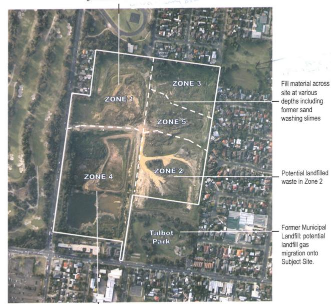
Existing quarry void: requires dewatering and backfilling
