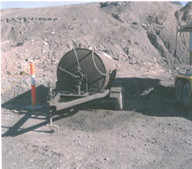
Fuel spill beneath a mobile fuel storage tank.
