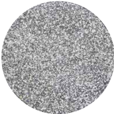
PAVING - TYPE 01 EXPOSED AGGREGATE CONCRETE
